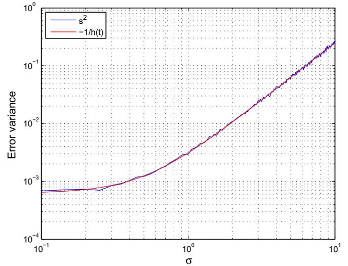
**Fig. 8.** The variance of the estimation error, i.e.,  $s^2$ , computed by Monte Carlo using  $10^3$  trials and the approximate variance based on the general theory for maximum likelihood estimators, i.e.,  $-1/h(t)$ , both as a function of standard deviation of the noise corrupting the data, i.e.,  $\sigma$ . Note that  $-1/h(t)$  accurately tracks  $s^2$  and both have a strong dependence on the noise in the original data, which is described by the standard deviation  $\sigma$ .
